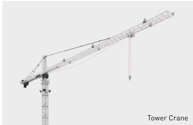
Luffing Jib Crane
